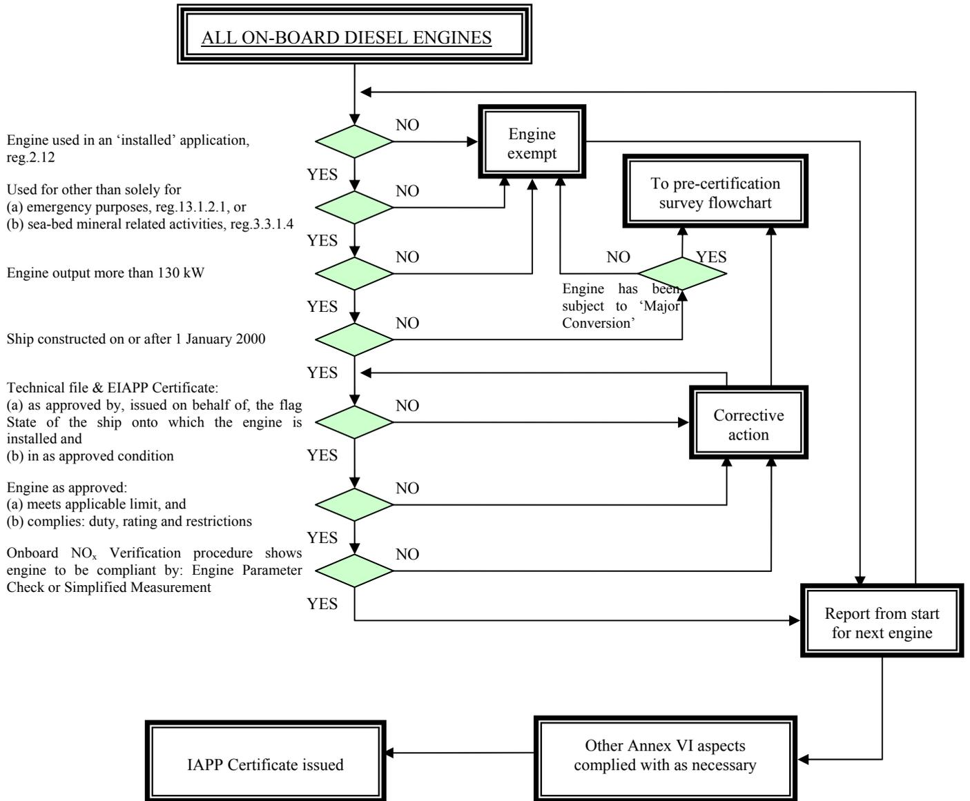
Figure 2 – Initial survey on board a ship
